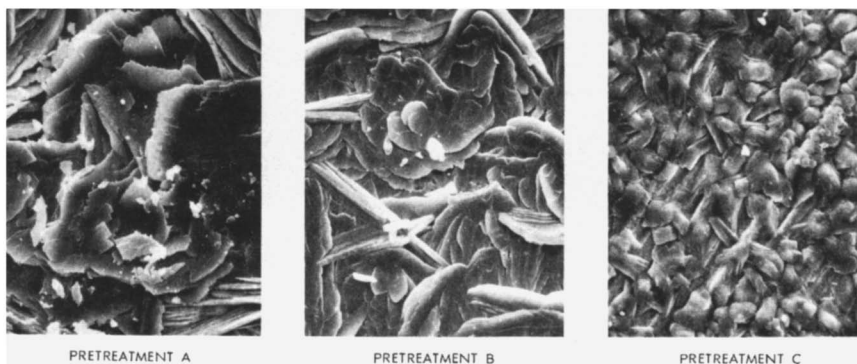
Figure 2. Phosphated surfaces before electrodeposition ( \times 450 )
